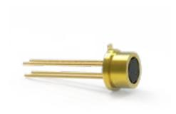
MTP10-B7F55 TSR infrared thermopile temperature sensor is a non-contact temperature sensor with a temperature measurement field of view of up to 76°. It has a built-in MEMS thermopile chip and adopts the 8~14 $\mu$ m bandpass filter exclusively customized by MFrontier. The average transmittance is  $\geq$  75%. It has the characteristics of high precision NTC and can be widely used in a variety of temperature measurement fields.
