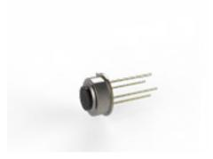
The MTP10-A6LF55 infrared thermopile temperature sensor is a noncontact temperature sensor with a temperature measurement field of view of up to 18°. It has a built-in MEMS thermopile chip and adopts the 8~14µm bandpass filter exclusively customized by MFrontier. The average transmittance is  $\geq$  75%. It has the characteristics of high-precision NTC and can be widely used in a variety of temperature measurement fields.
