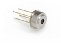
The MTP10-A6F55 infrared thermopile temperature sensor is a non-contact temperature sensor with a temperature measurement field of view of up to 62°. It has a built-in MEMS thermopile chip and adopts the 8~14 $\mu$ m bandpass filter exclusively customized by MFrontier. The average transmittance is  $\geq$  75%. It has the characteristics of High sensitivity NTC, and can be widely used in a variety of temperature measurement fields.
